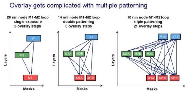
Masking pattern define the cost of chip making and as technology node move to lower nano meter technology cost would be much higher and newer lithography process such as EUV or E-Beam must pave wave for cost reduction as shown in table 1.
